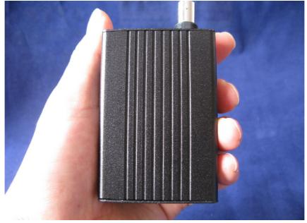
Most of the components of this kit are SMD parts and already pre-mounted by factory on PCB, so you will only need to solder about 20 through-hole parts including all the connectors and buttons. The case is custom made aluminum alloy case, with anodized finish and silkscreen printing. The whole kit will look like this:
