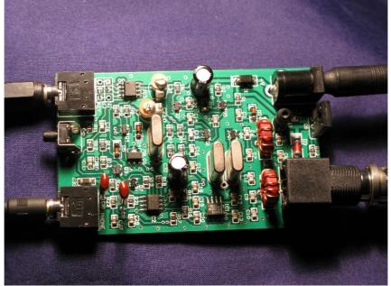
Direct conversion receiver with a 2-pole crystal filter in the front-end and an audio filter, plus typical 3 watts RF output power at 12 volt, it gives you enough chance to make some QSO's on 40 meter band. Now, two frequencies are offered: 7010 kHz or 7020 kHz, and 7025 kHz and 7030 kHz will follow shortly.
