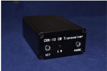
The RF output power is about 3 watt at 12V. Power supply range is 9-15V. TX current is about 500 mA, and RX current is about 15 mA (measured at 12V). The built-in MCU can generate side tone of about 700 Hz, switch RX/TX, and act as a keyer for not only paddle (normal paddle or bug key simulation mode), but also straight key.
