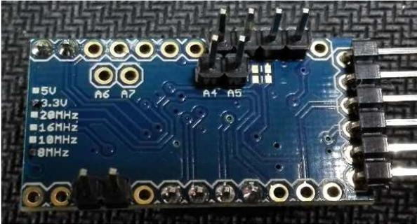
Install 4-pin header from GND to A3 on the bottom side.
