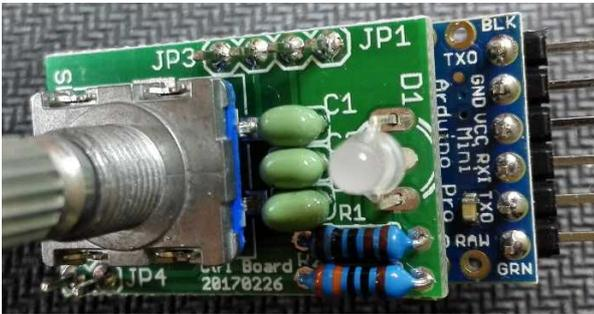
Stack up the Ctrl board from the top side of the Arduino board.
