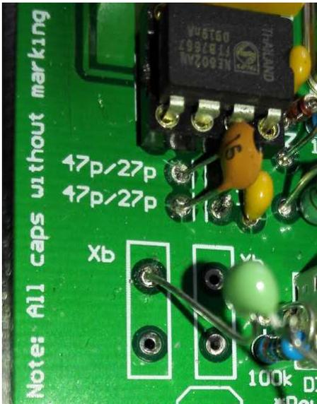
Use a 104 capacitor to connect JP9 (the pin on the right, GND on the left) to BFO (one pin of Xa' as shown), and another 104 to connect JP7 (the pin on the left, GND on the right) to VFO (one pin of Xb as shown). You can use a short wire to connect GND pin (JP8 left pin) to the ground of the main board for shorter and better grounding. As for 15pF capacitor, you can install near NE602 as shown to help improve spurs but it is optional here.
