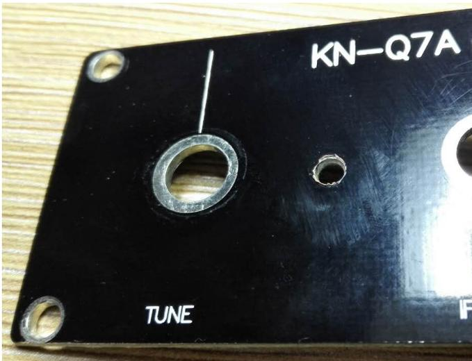
You will need to drill a 3mm diameter hole for LED in the middle of two holes for potentiometers.
