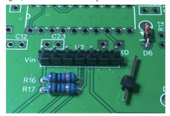
Plug in the 5351 module on the pin header and solder. The chip on the module might be a Chinese compatible chip with Silicon Labs SI5351, but it works just fine.
