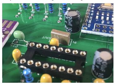
Populate all the parts L1-1uH, Q4-BS170, FL1-PFB455JR, U1-CD2003, C8,C9,C10,C21-100nF, C12,C17-10nF, C11-560pF or 620pF or 680pF, and C25-5.1pF and solder to complete the soldering of the main board.
