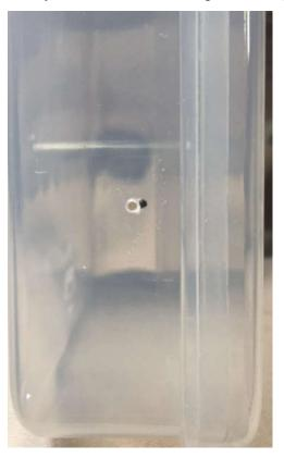
Press the board down so you can get correct locations for audio jacks, power supply jack and USB port on container sides, or the buttons will lift the board. Now mark the locations.
