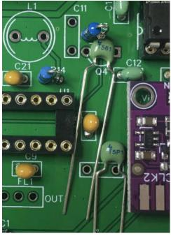
The photo shows the center pin of Q4-BS170 to make sure it is safe from static.
