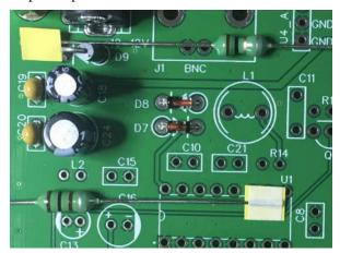
Solder L2, C13-10uF, C1, C16-100uF, C2, C14, C15-100nF. Beware of the polarity of C1, C13 and C16.
