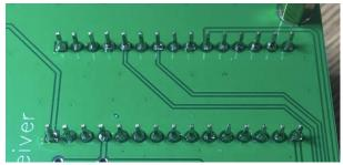
Now it is test time. Plug in the 12V power supply (center positive) and measure the voltage on the + pad of C1 - 100uF with the red probe. 4.93V falls well in the tolerance range of 5V regulator on the Nano module. Don't short circuit in this step, or the regulator will be damaged and it is very difficult to desolder the Nano module.
