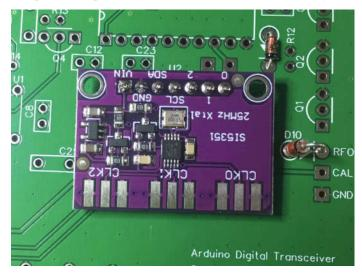
Turn the main board and solder the pin headers. Again, don't need to trim the extra leads.
